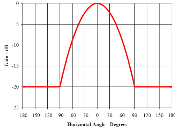
Figure 7.7.4-2 Simplified antenna pattern [ITU-R M.2135].
