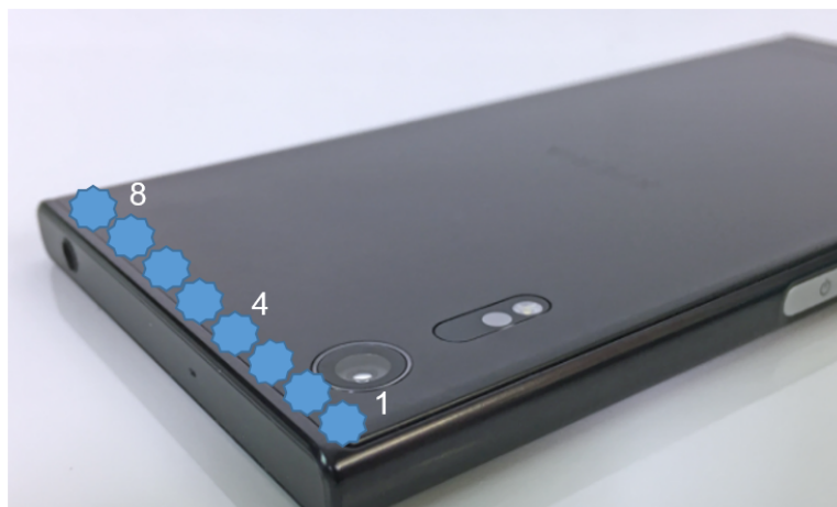
Figure 6.2.1.1.2-2: antenna arrangement on the UE used for the evaluation of beamforming gain.
