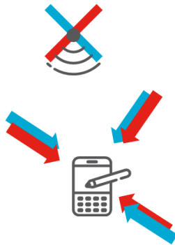
Figure D-1: received DL signal as a coherent sum of dual-polarized rays.
