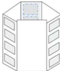
Figure A.2.1-2: Three sector antenna placement.
