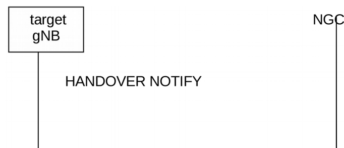
Figure 7.3.4.2.5-5: Example of Handover Notification procedure
