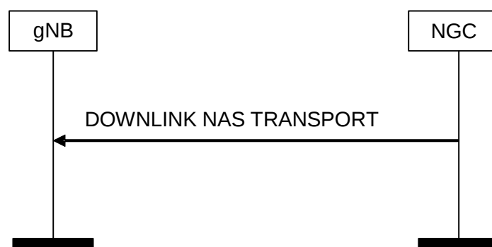
Figure 7.3.4.2.4-2: Example of Downlink NAS Transport procedure
