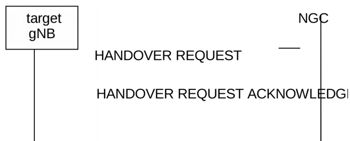
Figure 7.3.4.2.5-2: Example of Handover Preparation procedure
