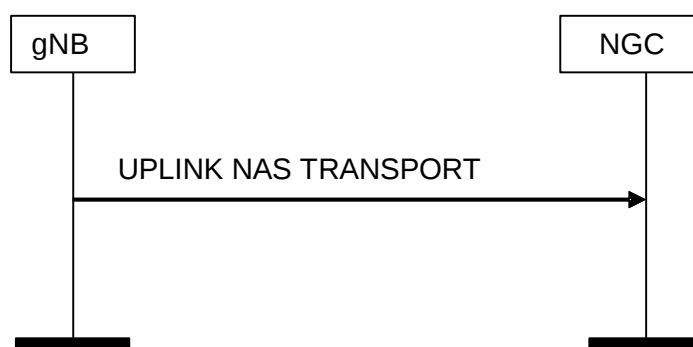
Figure 7.3.4.2.4-1: Example of Uplink NAS Transport procedure
