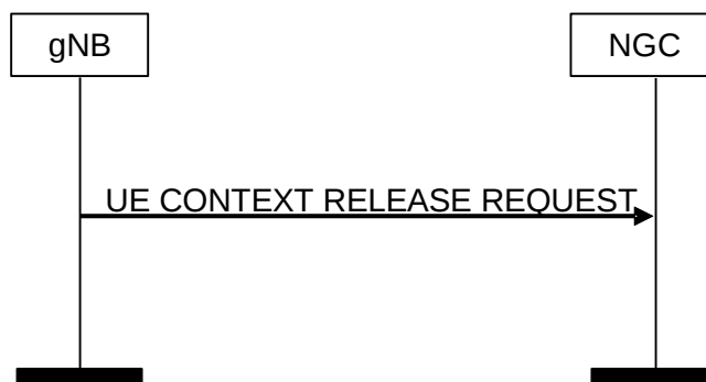
Figure 7.3.4.2.3-2: Example of UE Context Release Request procedure
