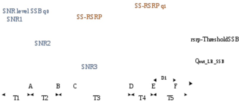
Figure 6.5.5.2.4-1: SNR and L1-RSRP variation for NR SA FR1 SSB-based beam failure detection and link recovery in DRX
