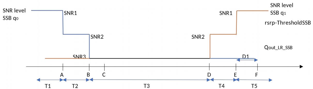
Figure 7.5.5.1.4-1: SNR variation SSB for NR SA FR2 SSB-based beam failure detection and link recovery in non-DRX
