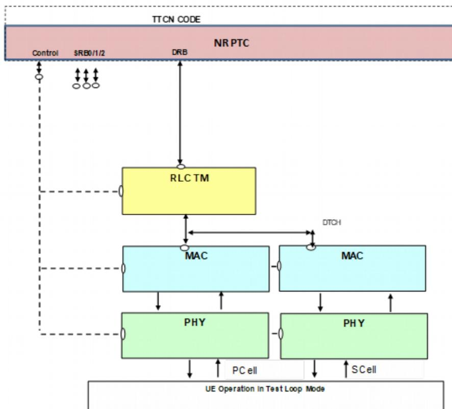
Figure 5.2.2.4.2-1: Test model for NR/5GC MAC CA testing
