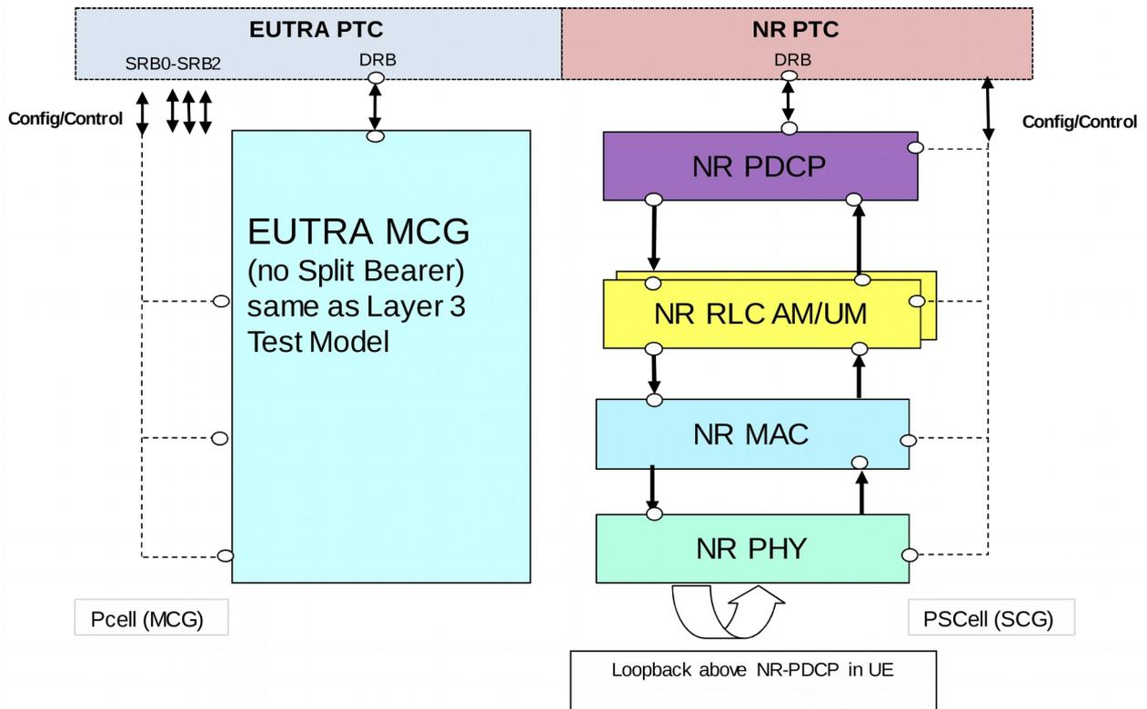
Figure 5.1.2.1-1: Test model for EN-DC PDCP testing (MN terminated MCG DRB and SN terminated SCG DRB)
