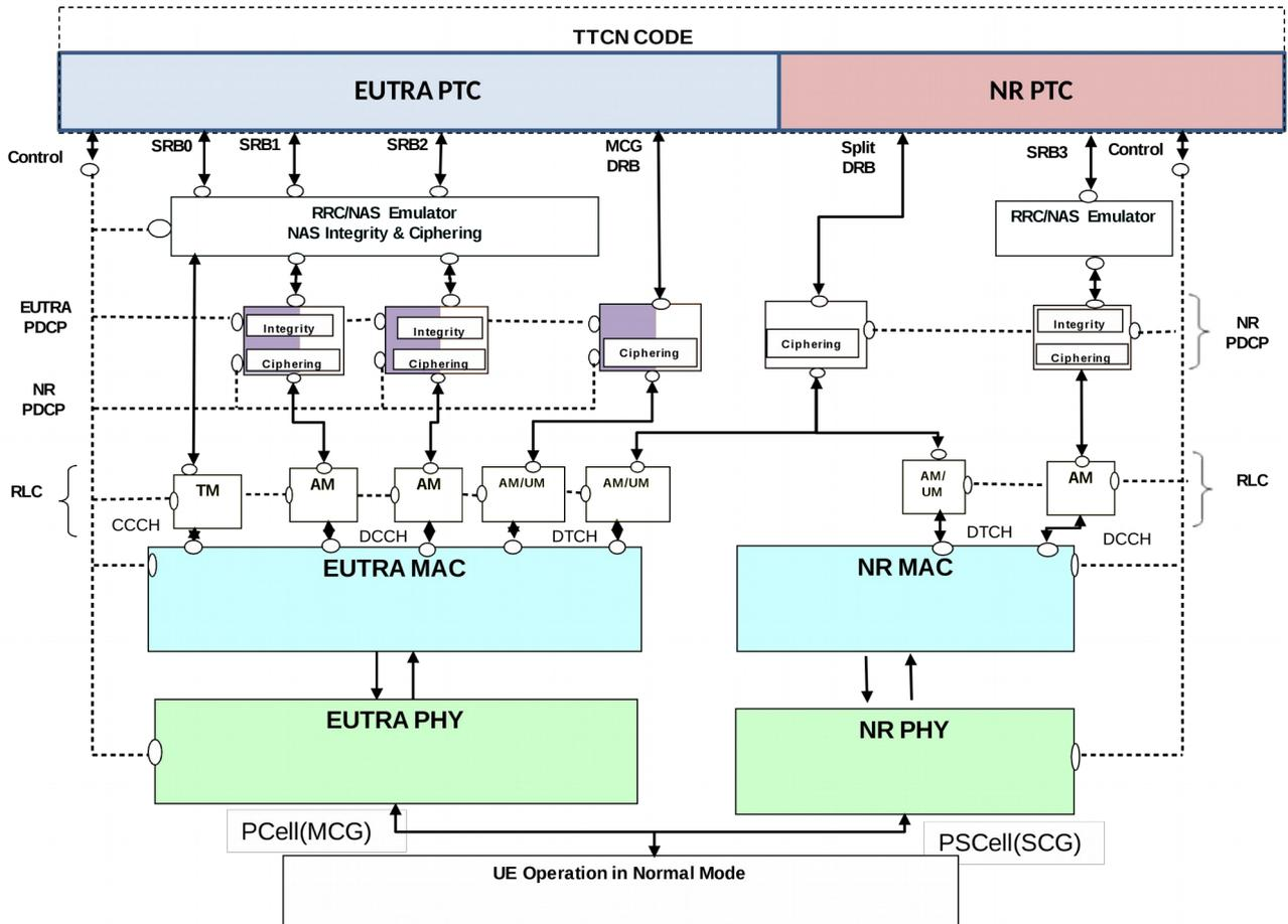
Figure 5.1.1.1-2: Test model for EN-DC Layer3 testing (MCG and split DRB)
