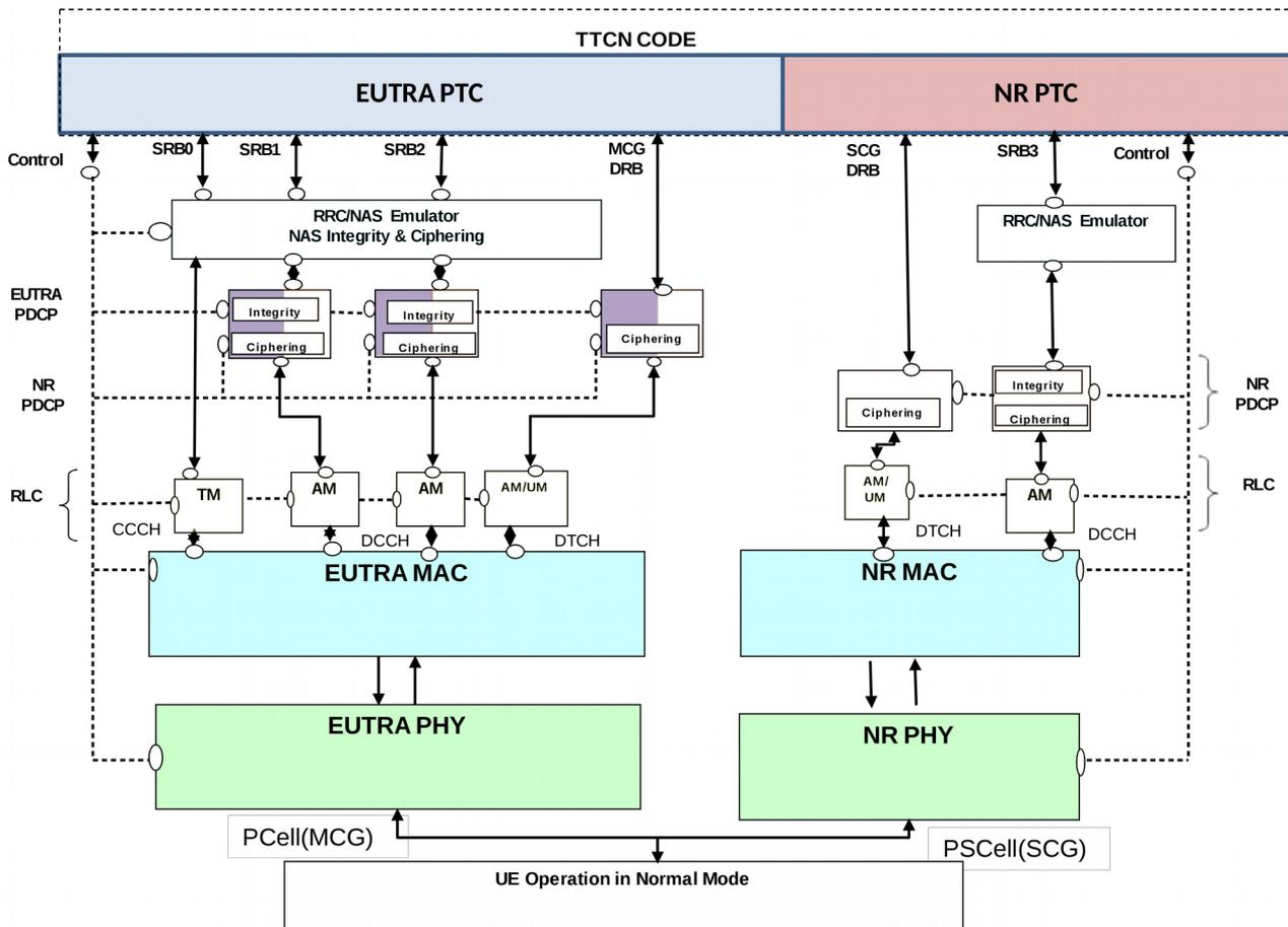
Figure 5.1.1.1-1: Test model for EN-DC Layer3 testing (MCG and SCG)
