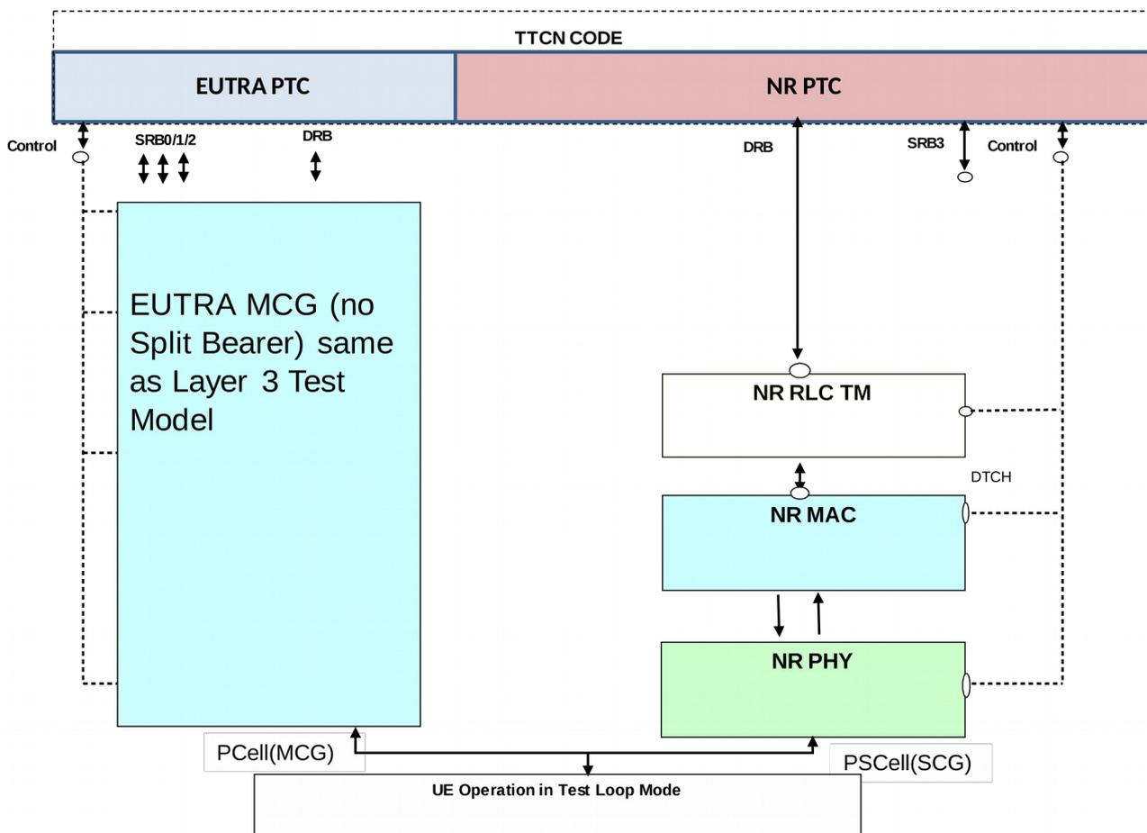
Figure 5.1.2.3.1-1: Test model for EN-DC MAC testing
