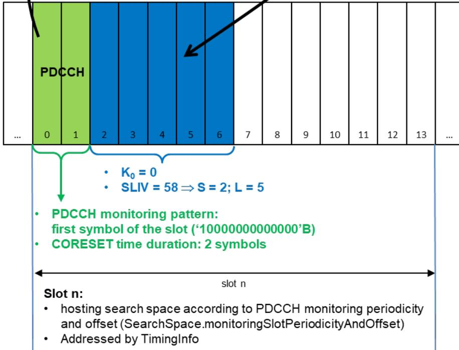
Figure 7.1.2.2-1: Example for time domain resource allocation for  $K_0 = 0$
