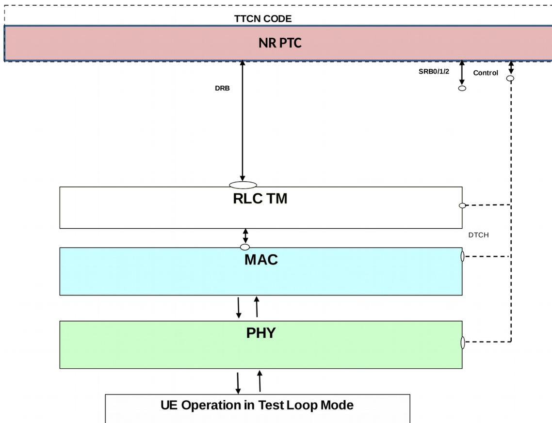
Figure 5.2.2.4.1-1: Test model for NR/5GC MAC testing
