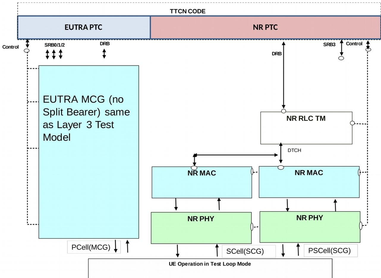
Figure 5.1.2.3.2-1: Test model for EN-DC MAC CA testing
