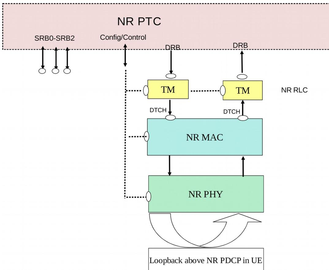
Figure 5.2.2.3-1: Test model for NR/5GC RLC testing
