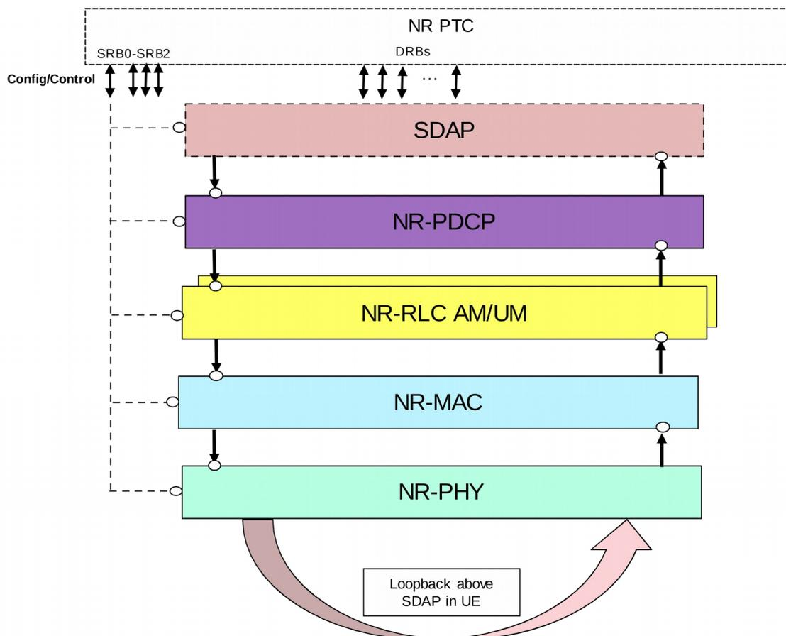
**Figure 5.2.2.1-1: Test model for NR/5GC SDAP testing**
