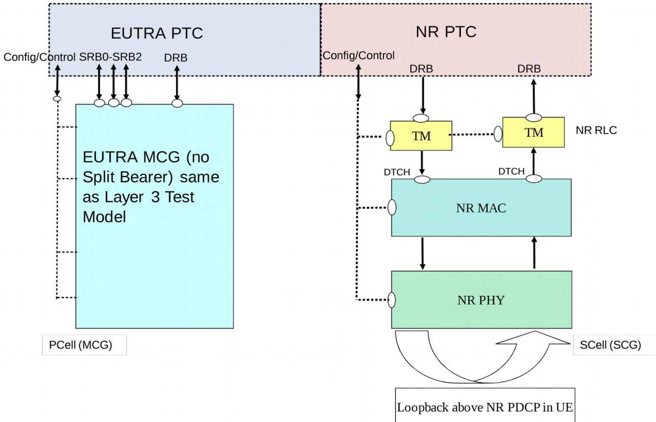
Figure 5.1.2.2-1: Test model for EN-DC RLC AM/UM testing
