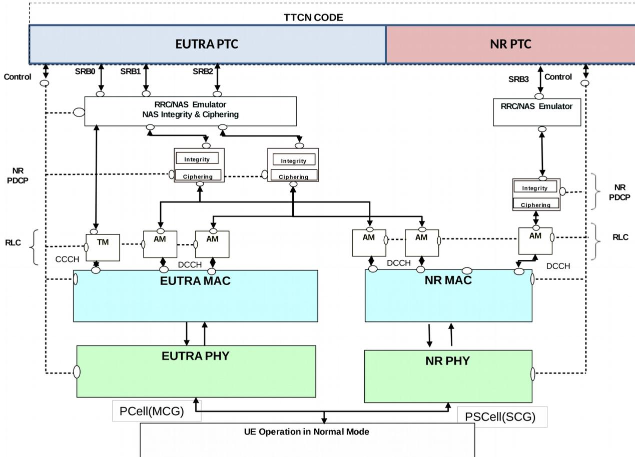
Figure 5.1.1.1-3: Test model for EN-DC Layer3 testing (Split SRB(s), DRBs removed for clarity)
