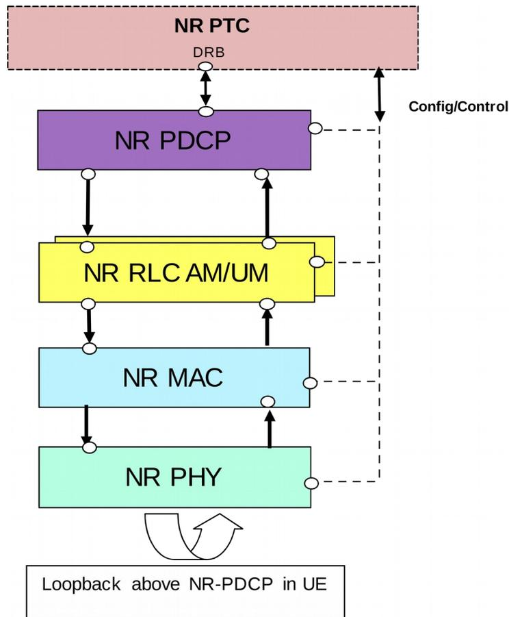
**Figure 5.2.2.2-1: Test model for NR/5GC PDCP testing**
