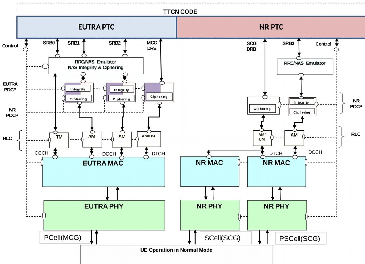
Figure 5.1.1.2-1: Test model for EN-DC Layer3 CA testing
