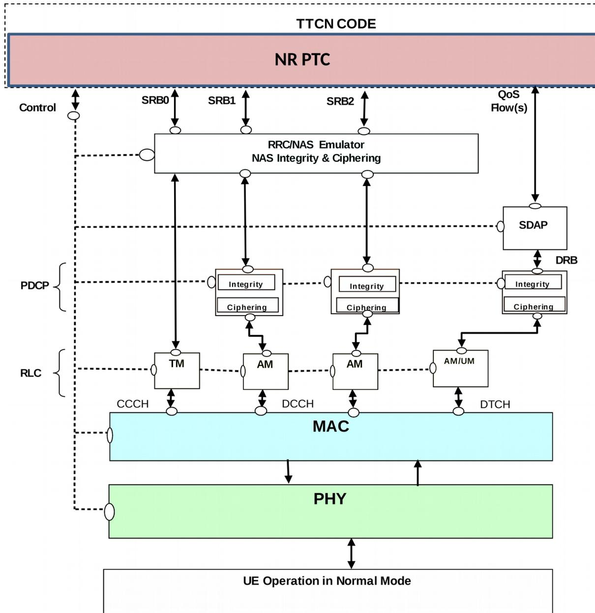
Figure 5.2.1.1-1: Test model for NR/5GC Layer3 testing
