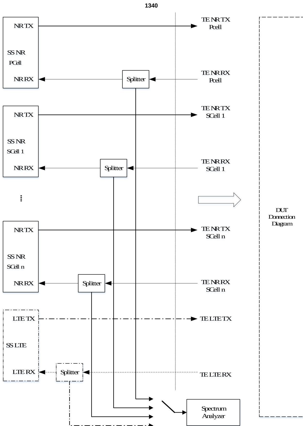
Figure A.3.1.2.3: Test Equipment connection for NR CA TX-tests with additional Spectrum Analyser
