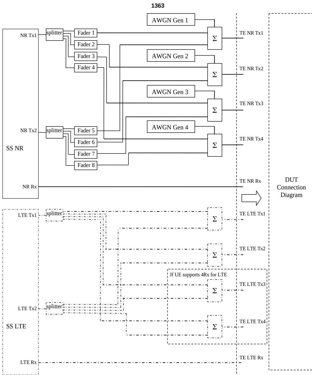
**Figure A.3.1.7.4: Test Equipment connection for Demodulation Performance and CSI reporting tests with antenna configuration 2x4**
