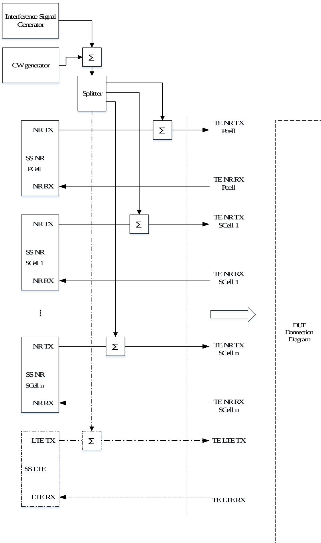
**Figure A.3.1.4.7: Test Equipment connection for NR CA Receiver tests with additional Modulated Interference signal and/or CW Interference signal**
