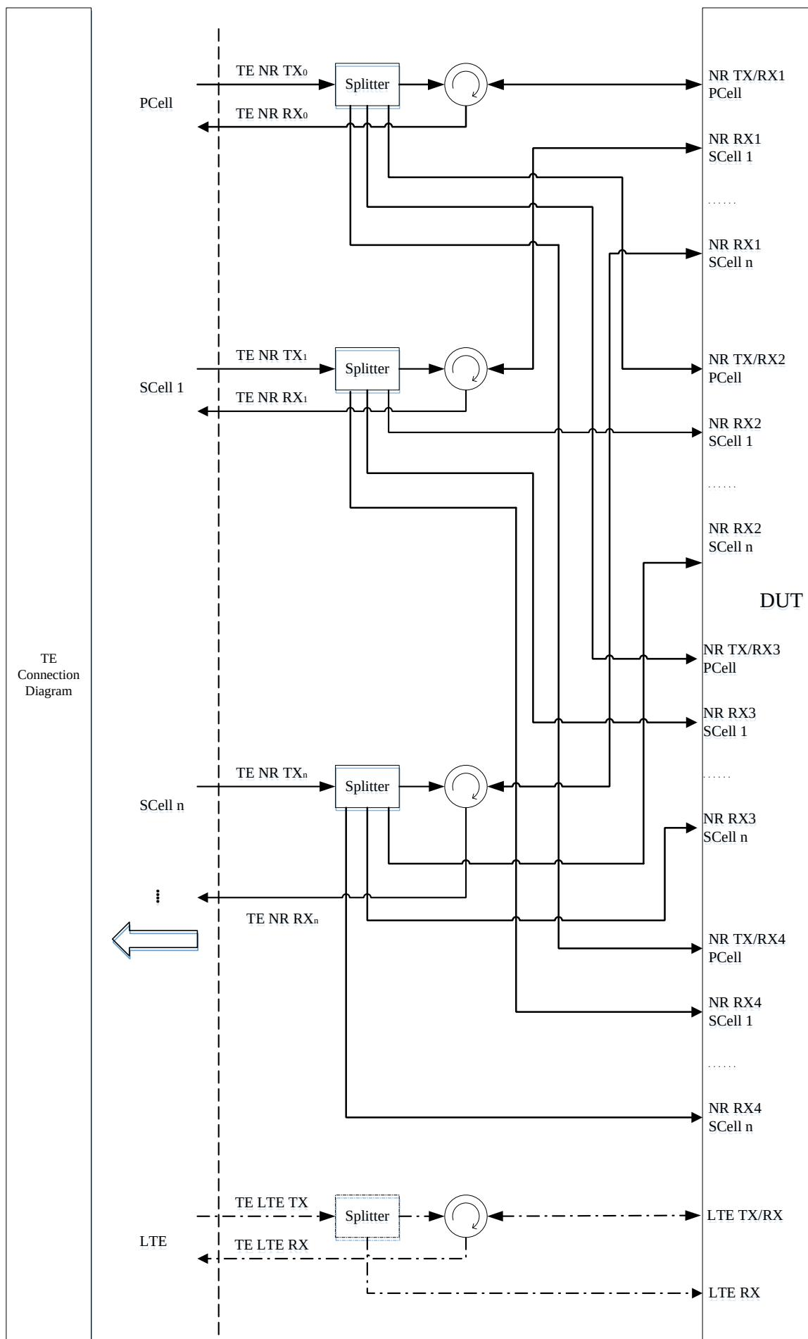
**Figure A.3.2.6.2: User Equipment connection for UEs with NR CA and NR 4Rx (component carriers on separated connectors) and LTE**
