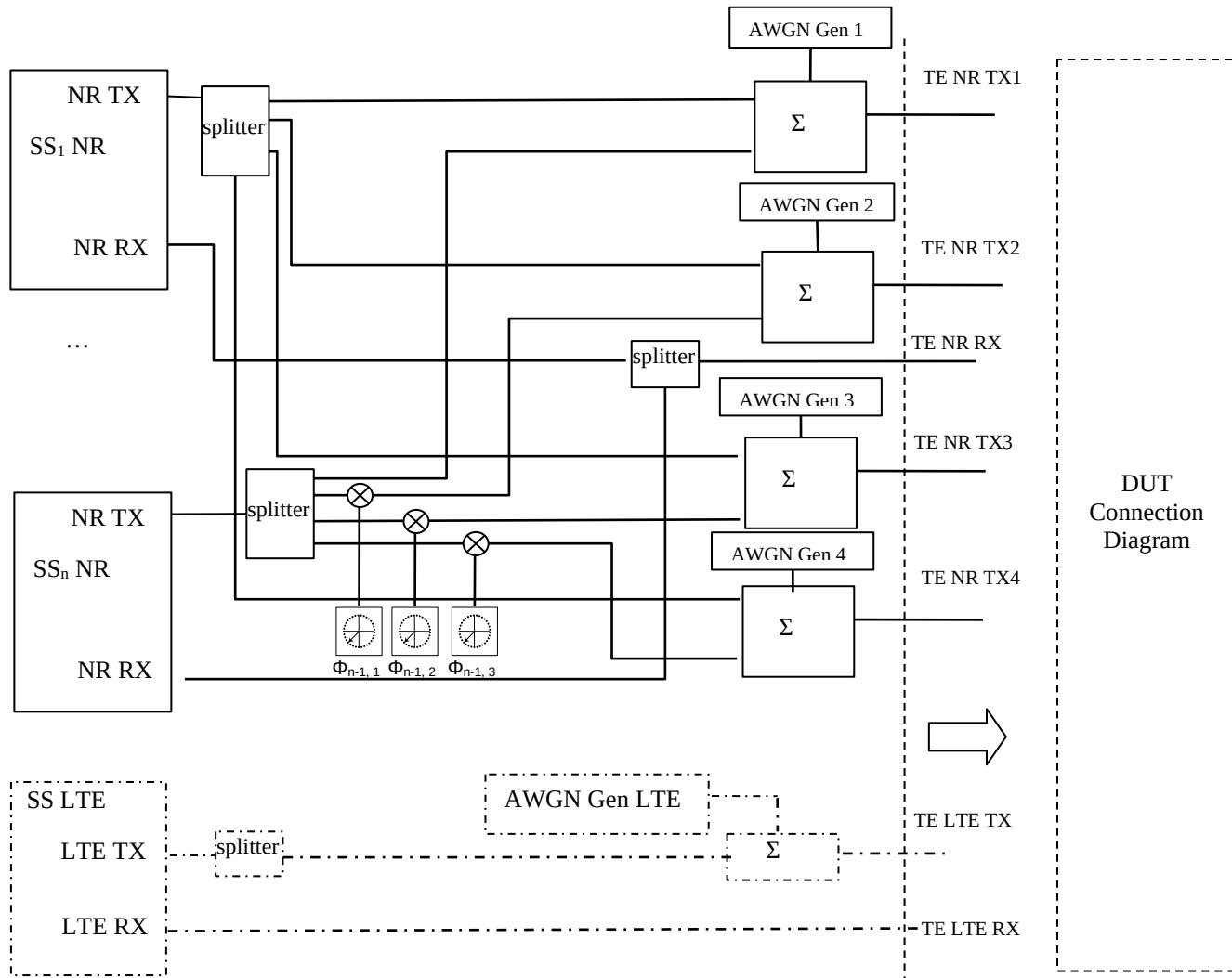
Figure A.3.1.8.5: Test Equipment connection for tests with more than one NR cell and antenna configuration 1x4
