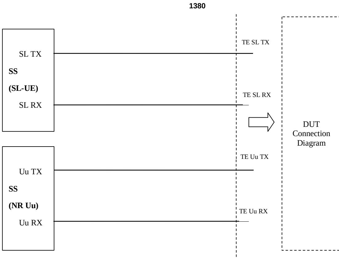
**Figure A.3.1.9.3: Test Equipment connection for inter-band con-current NR V2X operation**
