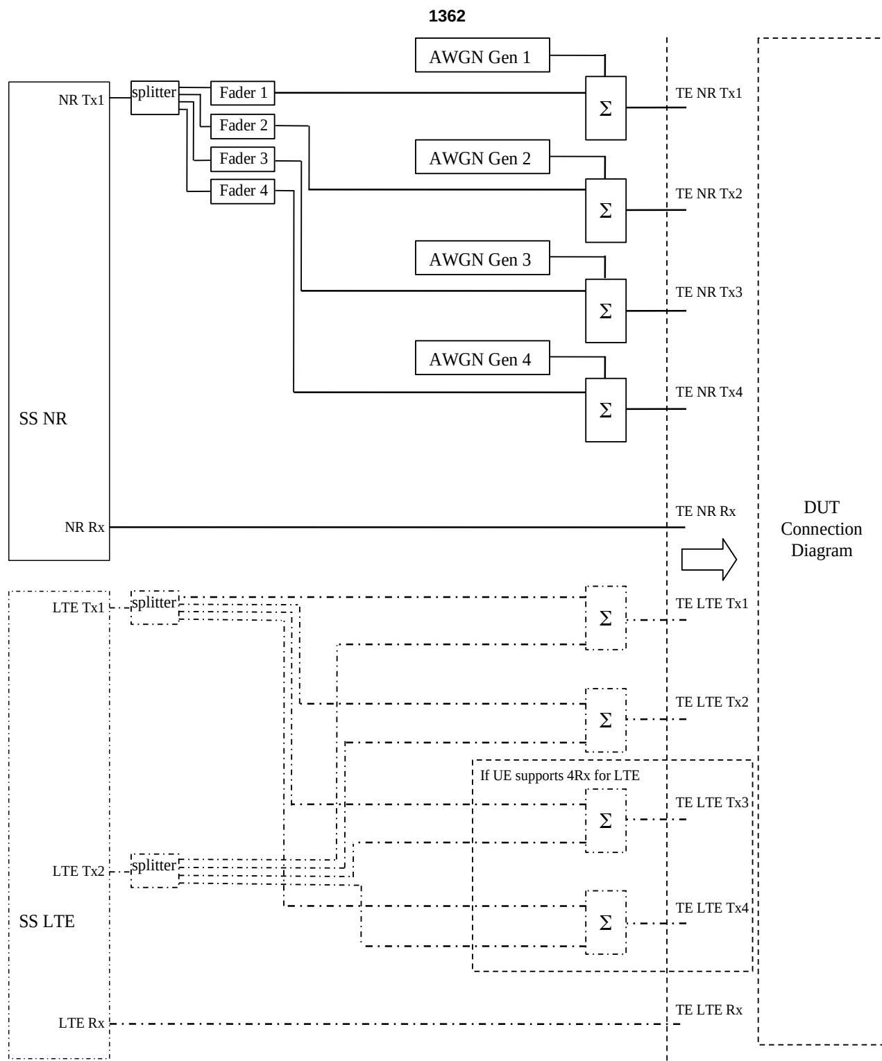
**Figure A.3.1.7.3: Test Equipment connection for Demodulation Performance and CSI reporting tests with antenna configuration 1x4**
