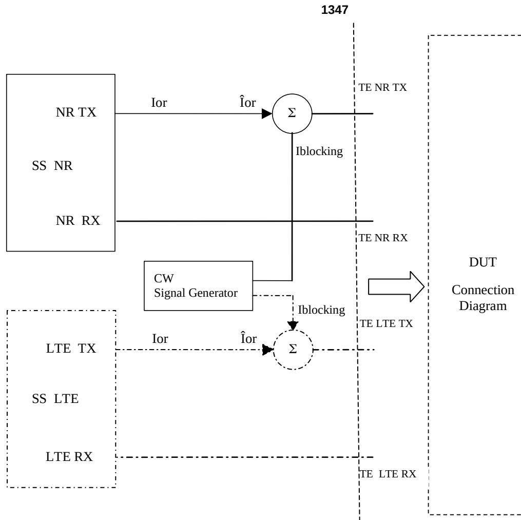
**Figure A.3.1.4.2: Test Equipment connection for Receiver tests with CW Interference**
