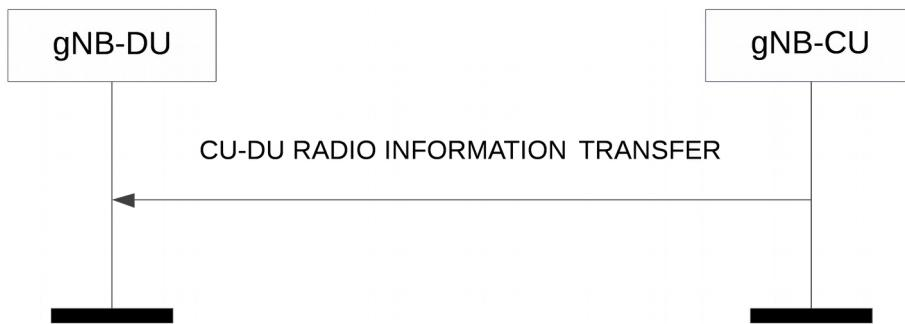
**Figure 8.9.2.2-1: CU-DU Radio Information Transfer procedure.**
