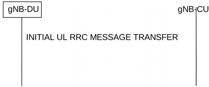
**Figure 8.4.1.2-1: Initial UL RRC Message Transfer procedure.**
