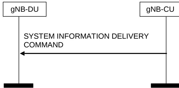
**Figure 8.6.1.2-1: System Information Delivery procedure. Successful operation.**
