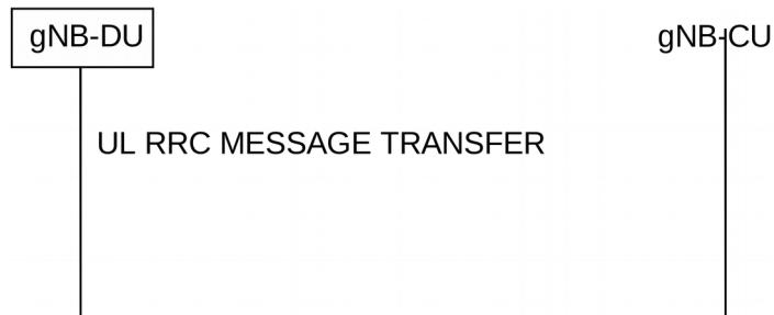
**Figure 8.4.3.2-1: UL RRC Message Transfer procedure**
