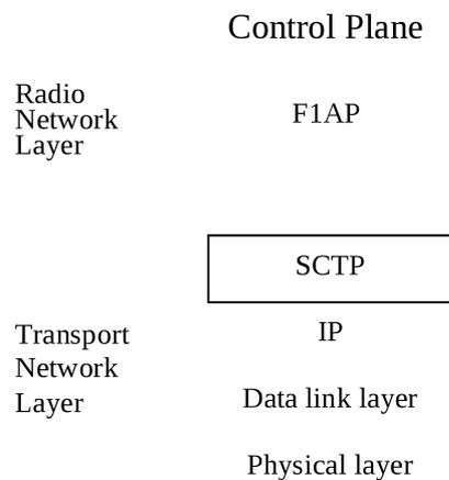
**Figure 7.1-1: Interface protocol structure for F1-C**
