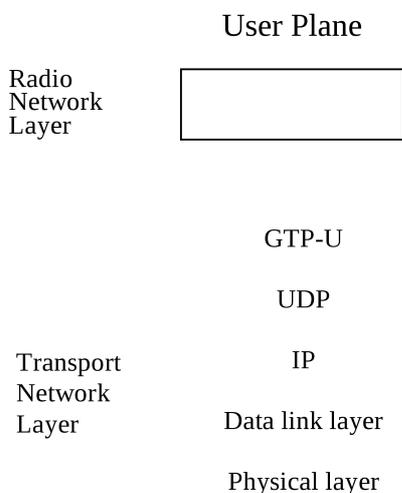
**Figure 7.2-1: Interface protocol structure for F1-U**
