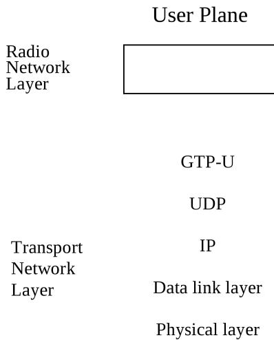
**Figure 7.2-1: Interface protocol structure for F1-U**
