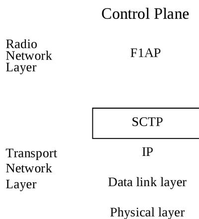
**Figure 7.1-1: Interface protocol structure for F1-C**
