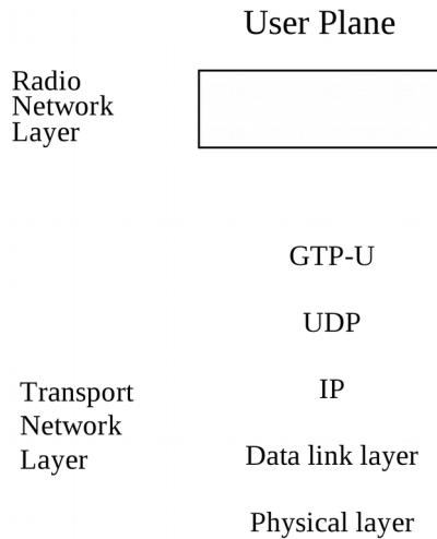
**Figure 7.2-1: Interface protocol structure for F1-U**
