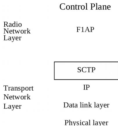
**Figure 7.1-1: Interface protocol structure for F1-C**
