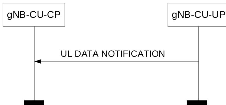
**Figure 8.3.10.2-1: UL Data Notification procedure: Successful Operation.**
