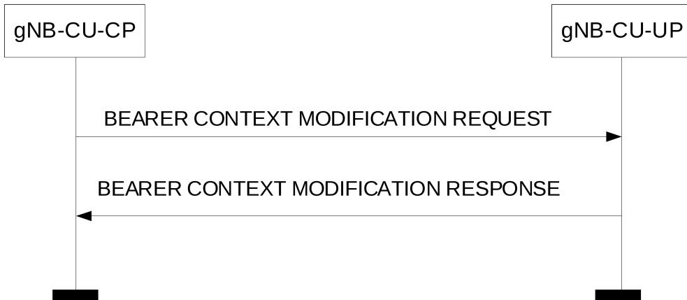
**Figure 8.3.2.2-1: Bearer Context Modification procedure: Successful Operation.**
