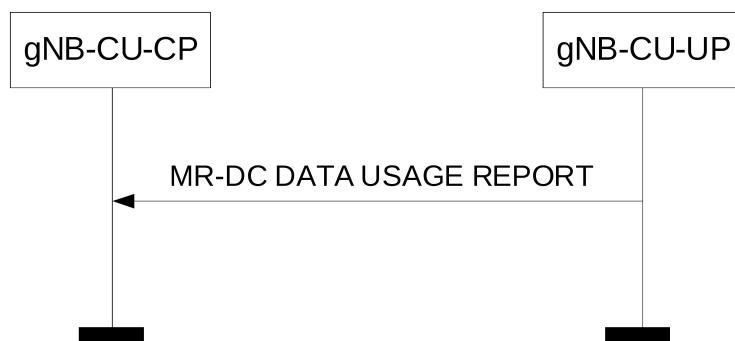
**Figure 8.3.11.2-1: MR-DC Data Usage Report procedure: Successful Operation.**
