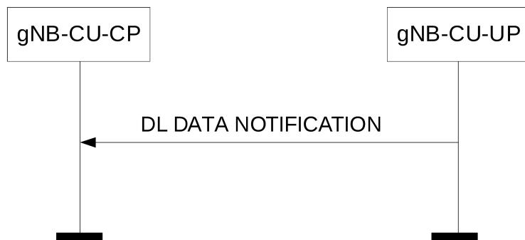
**Figure 8.3.7.2-1: DL Data Notification procedure: Successful Operation.**
