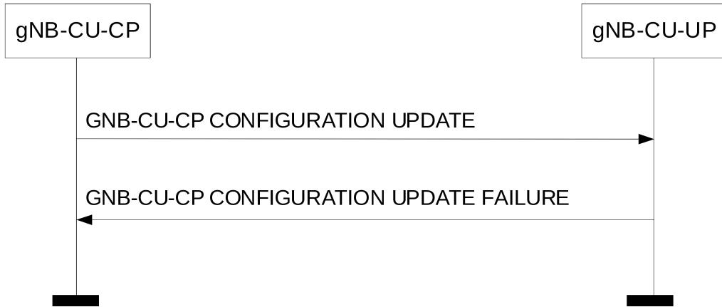
**Figure 8.2.6.3-1: gNB-CU-CP Configuration Update procedure: Unsuccessful Operation.**
