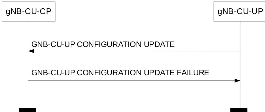
**Figure 8.2.5.3-1: gNB-CU-UP Configuration Update procedure: Unsuccessful Operation.**
