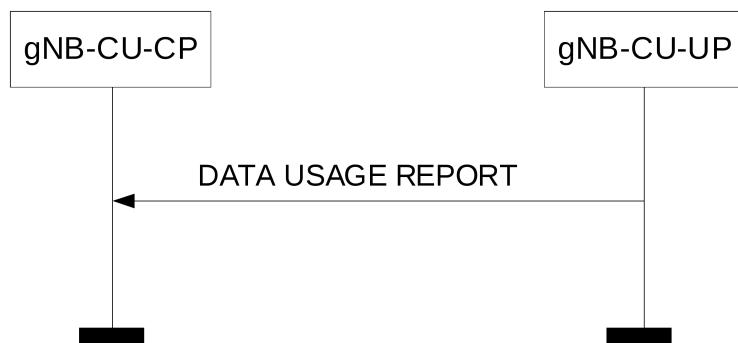
**Figure 8.3.8.2-1: Data Usage Report procedure: Successful Operation.**
