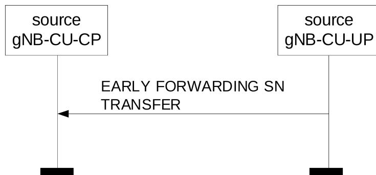
**Figure 8.3.12.2-1: Early Forwarding SN Transfer procedure: Successful Operation.**
