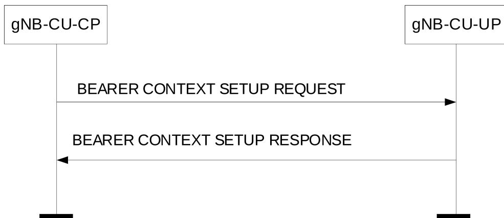
**Figure 8.3.1.2-1: Bearer Context Setup procedure: Successful Operation.**
