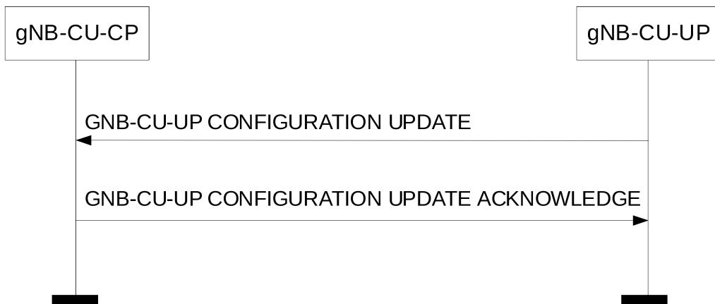
**Figure 8.2.5.2-1: gNB-CU-UP Configuration Update procedure: Successful Operation.**
