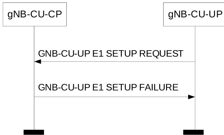
**Figure 8.2.3.3-1: gNB-CU-UP E1 Setup procedure: Unsuccessful Operation.**
