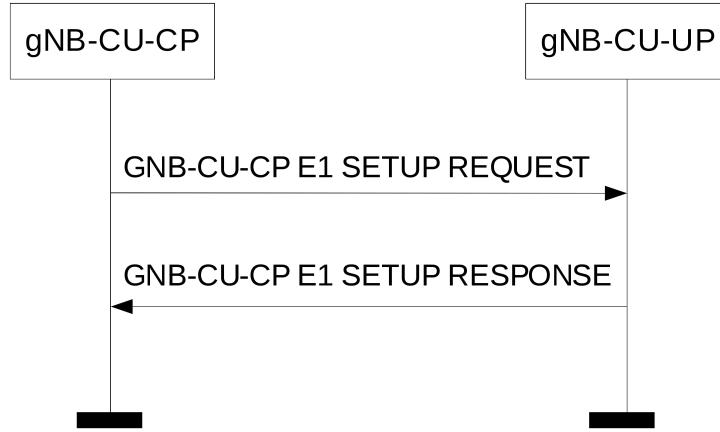
**Figure 8.2.4.2-1: gNB-CU-CP E1 Setup procedure: Successful Operation.**
