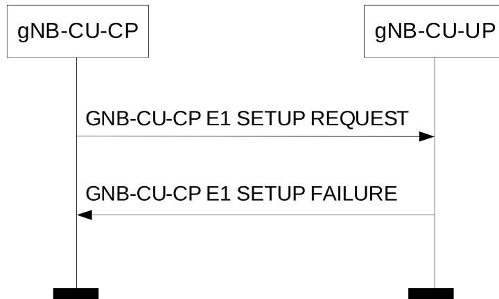
**Figure 8.2.4.3-1: gNB-CU-CP E1 Setup procedure: Unsuccessful Operation.**
