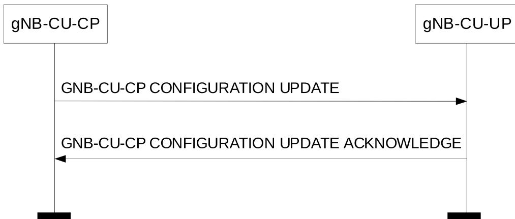
**Figure 8.2.6.2-1: gNB-CU-CP Configuration Update procedure: Successful Operation.**
