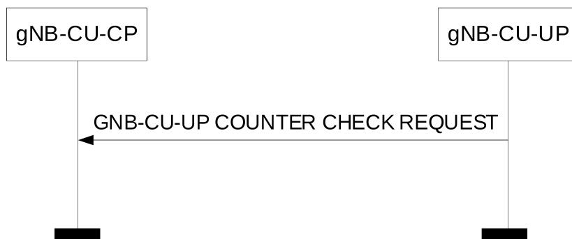
**Figure 8.3.9.2-1: gNB-CU-UP Counter Check procedure, successful operation.**
