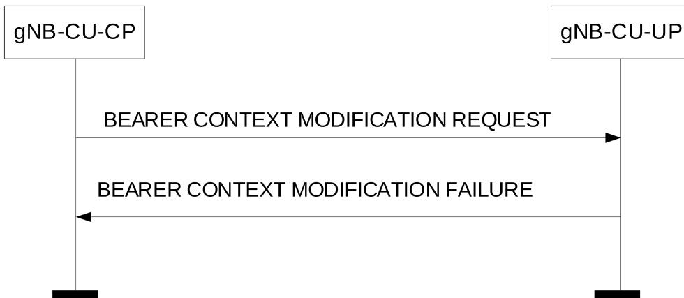
**Figure 8.3.2.3-1: Bearer Context Modification procedure: Unsuccessful Operation.**
