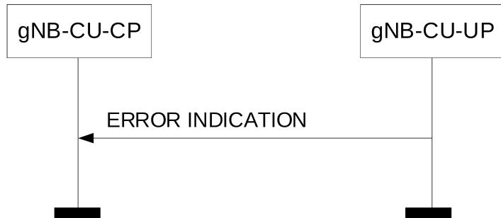
**Figure 8.2.2.2-2: Error Indication procedure, gNB-CU-UP originated. Successful operation.**
