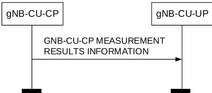
**Figure 8.3.x.2-1: GNB-CU-CP Measurement Results Information procedure. Successful operation.**
