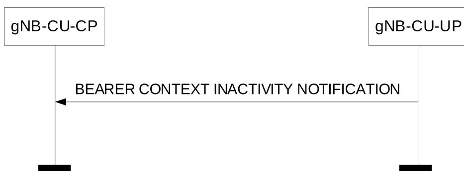
**Figure 8.3.6.2-1: Bearer Context Inactivity Notification procedure: Successful Operation.**
