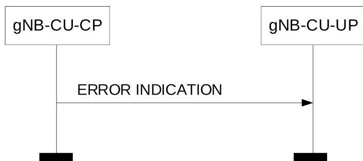
**Figure 8.2.2.2-1: Error Indication procedure, gNB-CU-CP originated. Successful operation.**
