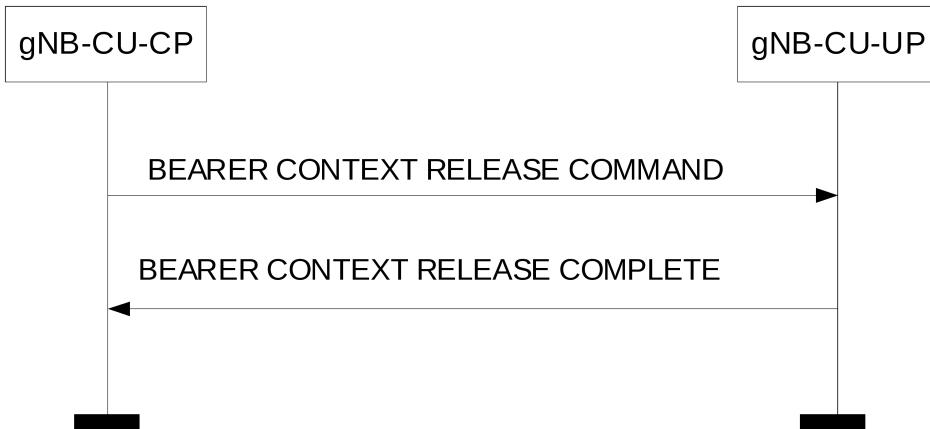
**Figure 8.3.4.2-1: Bearer Context Release procedure: Successful Operation.**
