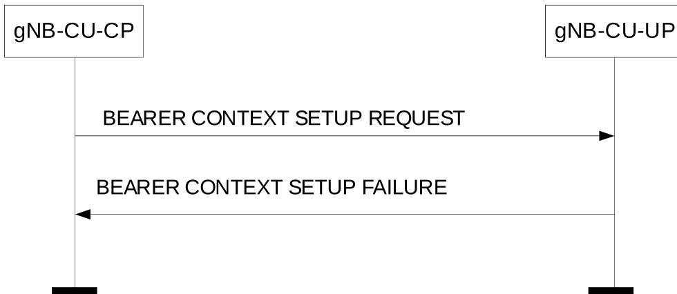
**Figure 8.3.1.3-1: Bearer Context Setup procedure: Unsuccessful Operation.**
