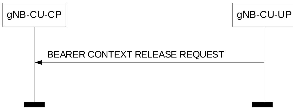
**Figure 8.3.5.2-1: Bearer Context Release Request procedure: Successful Operation.**
