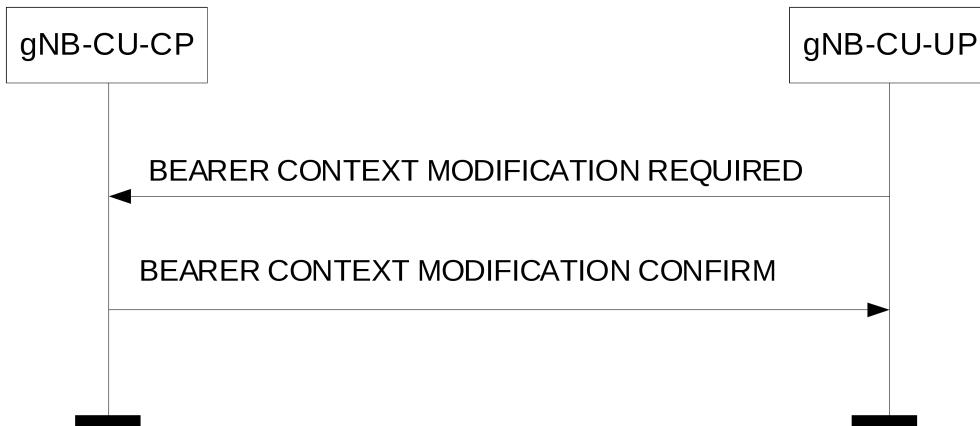
**Figure 8.3.3.2-1: Bearer Context Modification Required procedure: Successful Operation.**
