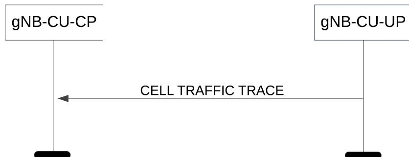
**Figure 8.4.3.2-1: Cell Traffic Trace procedure. Successful operation.**
