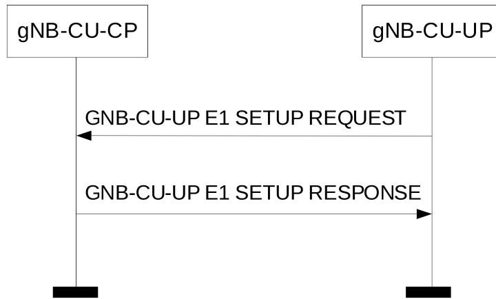
**Figure 8.2.3.2-1: gNB-CU-UP E1 Setup procedure: Successful Operation.**
