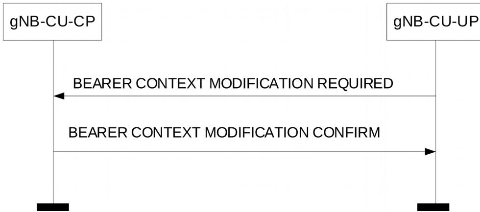
**Figure 8.3.3.2-1: Bearer Context Modification Required procedure: Successful Operation.**
