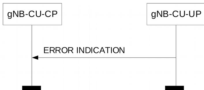
**Figure 8.2.2.2-2: Error Indication procedure, gNB-CU-UP originated. Successful operation.**
