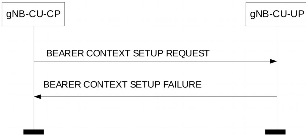
**Figure 8.3.1.3-1: Bearer Context Setup procedure: Unsuccessful Operation.**
