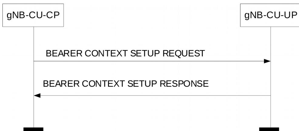
**Figure 8.3.1.2-1: Bearer Context Setup procedure: Successful Operation.**
