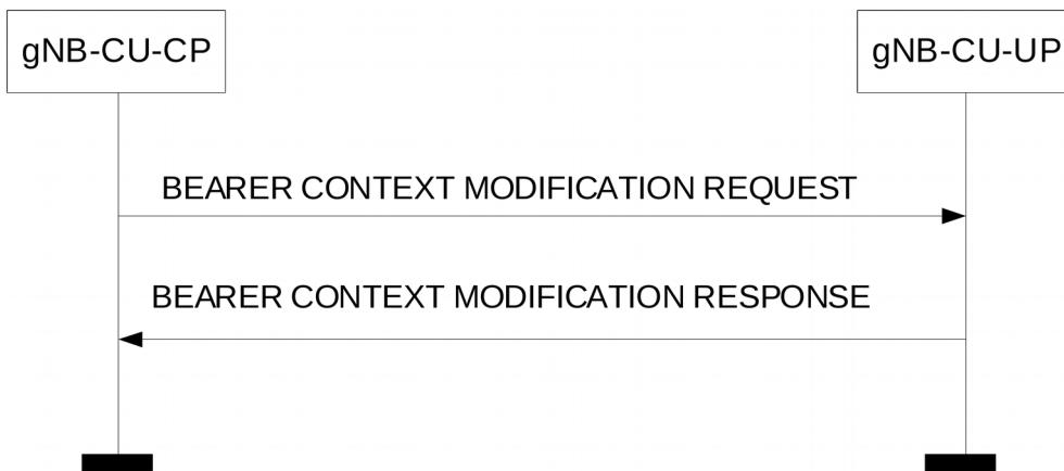
**Figure 8.3.2.2-1: Bearer Context Modification procedure: Successful Operation.**
