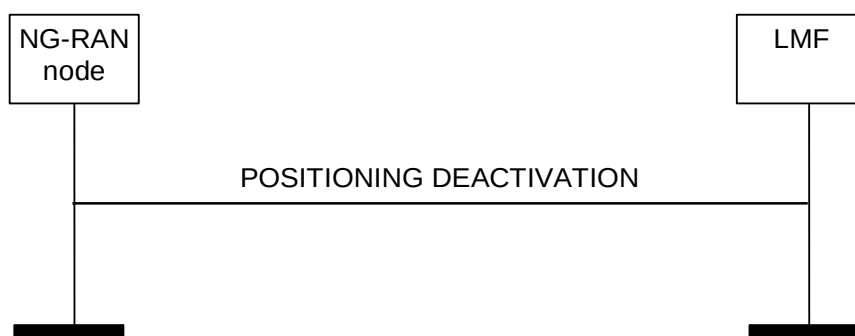
Figure 8.2.10.2-1: Positioning Deactivation procedure, successful operation
