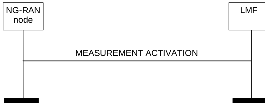
Figure 8.2.13.2-1: Measurement Activation procedure, successful operation
