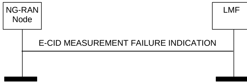
Figure 8.2.2.2-1: E-CID Measurement Failure Indication, successful operation
