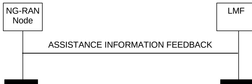
Figure 8.4.2.2-1: Assistance Information Feedback procedure
