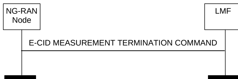
Figure 8.2.4.2-1: E-CID Measurement Termination procedure, successful operation
