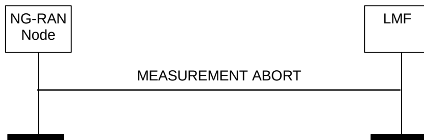
Figure 8.5.4.2.1: Measurement Abort Procedure: Successful Operation.
