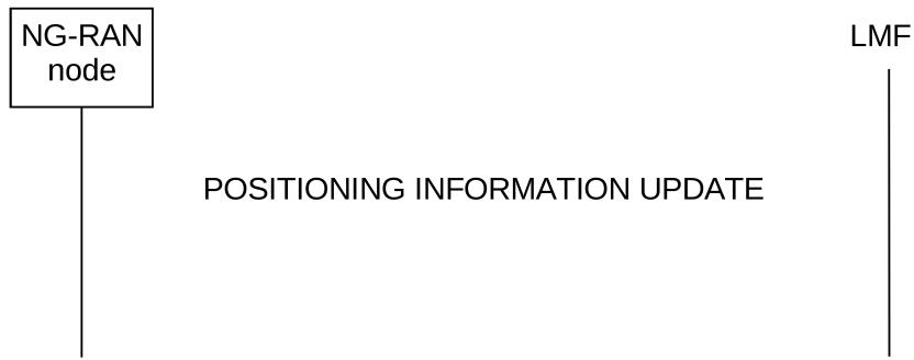
**Figure 8.2.7.2-1: Positioning Information Update procedure, successful operation**
