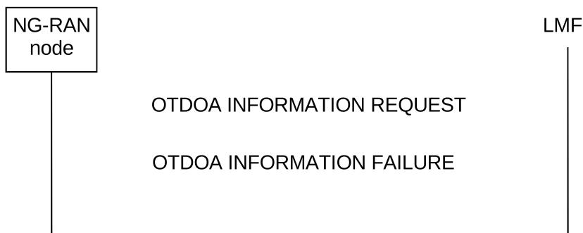
**Figure 8.2.5.3-1: OTDOA Information Exchange procedure, unsuccessful operation**
