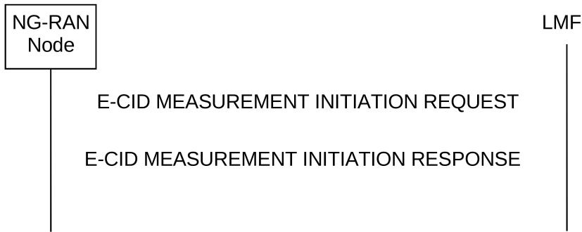
**Figure 8.2.1.2-1: E-CID Measurement Initiation procedure, successful operation**
