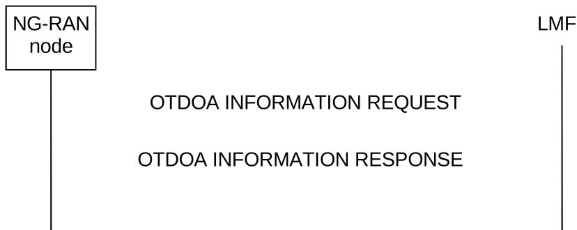
**Figure 8.2.5.2-1: OTDOA Information Exchange procedure, successful operation**
