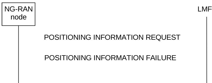
**Figure 8.2.6.3-1: Positioning Information Exchange procedure, unsuccessful operation**
