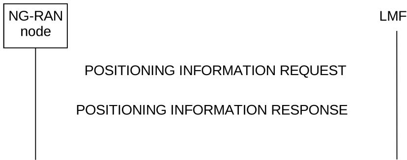
**Figure 8.2.6.2-1: Positioning Information Exchange procedure, successful operation**
