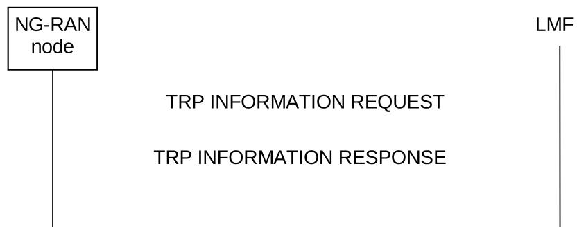
**Figure 8.2.8.2-1: TRP Information Exchange procedure, successful operation**
