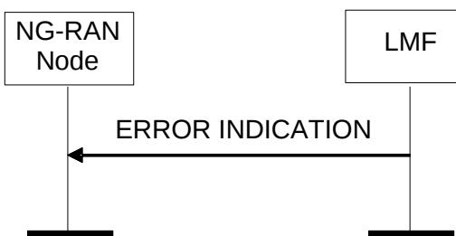
**Figure 8.3.1.2-1: Error Indication procedure, LMF originated, successful operation**
