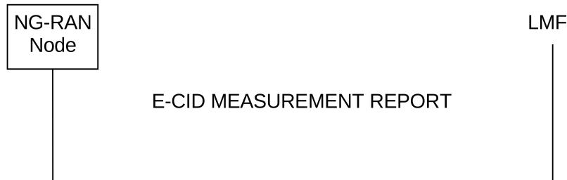
**Figure 8.2.3.2-1: E-CID Measurement Report procedure, successful operation**
