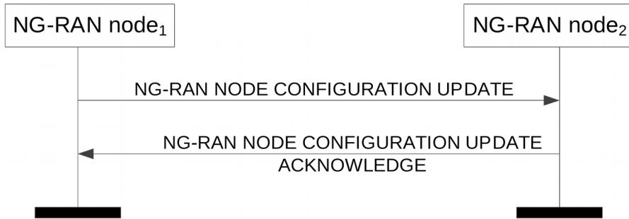
**Figure 8.4.2.2-1: NG-RAN node Configuration Update, successful operation**
