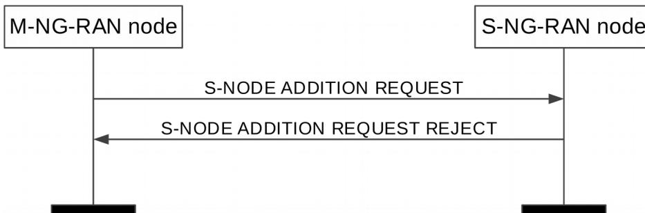
Figure 8.3.1.3-1: S-NG-RAN node Addition Preparation, unsuccessful operation
