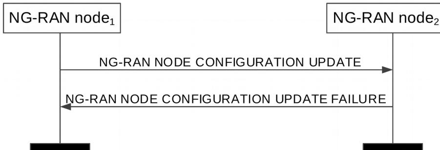
**Figure 8.4.2.3-1: NG-RAN node Configuration Update, unsuccessful operation**
