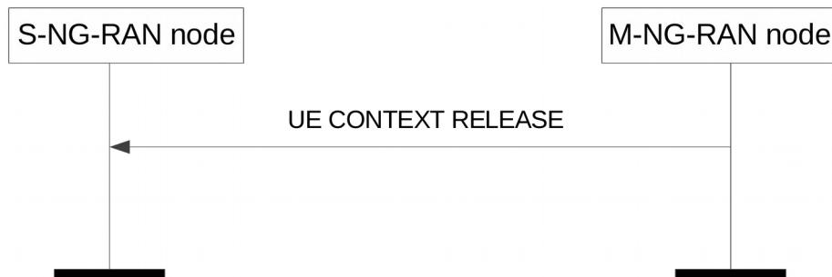
**Figure 8.2.7.2-2: UE Context Release, successful operation for dual connectivity**
