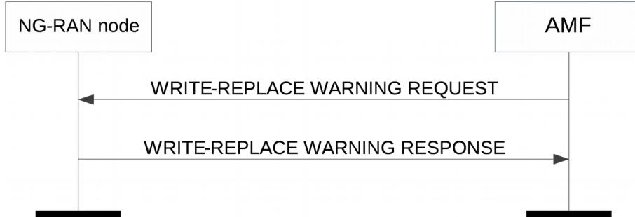
**Figure 8.9.1.2-1: Write-Replace Warning procedure: successful operation**
