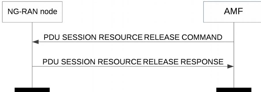
**Figure 8.2.2.2-1: PDU session resource release: successful operation**
