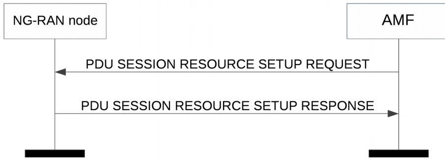
**Figure 8.2.1.2-1: PDU session resource setup: successful operation**
