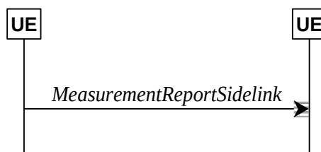
Figure 5.8.10.5.1-1: NR sidelink measurement reporting
