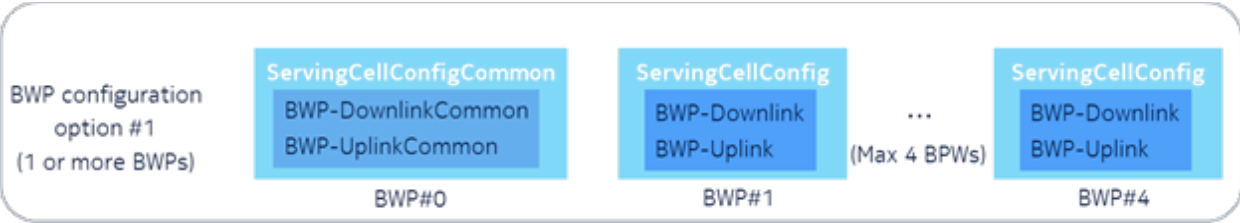
Figure B2-1: BWP#0 configuration without dedicated configuration
