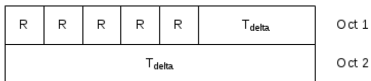
Figure 6.1.3.21-1: Timing Delta MAC CE
