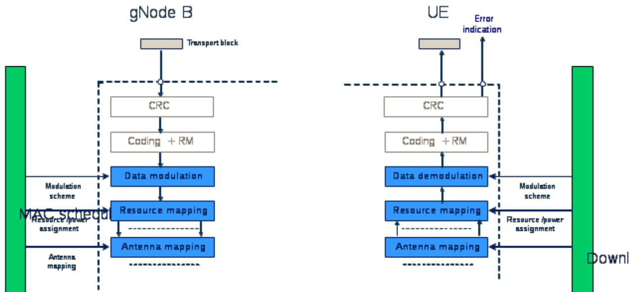
Figure 5.2.3-1: Physical-layer model for PCH transmission
