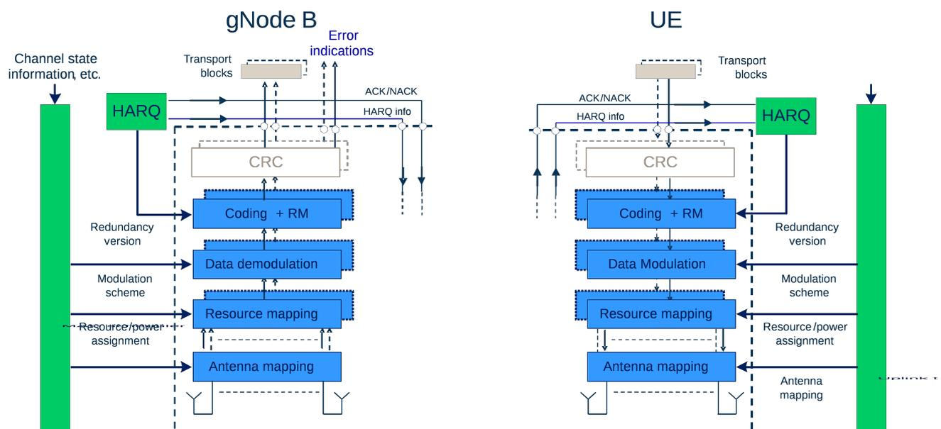
Figure 5.1.1-1: Physical-layer model for UL-SCH transmission
