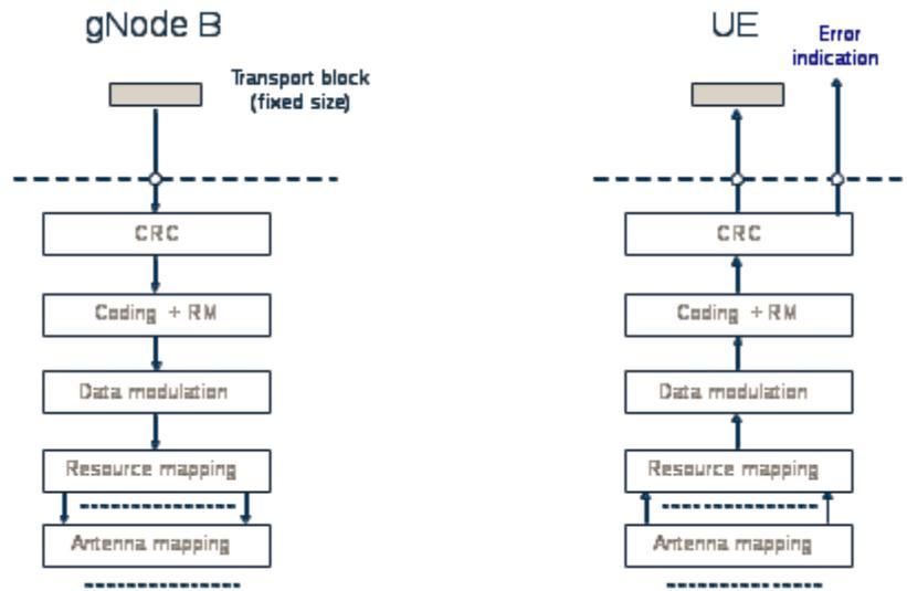
Figure 5.2.2-1: Physical-layer model for BCH transmission
