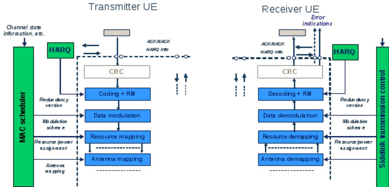
Figure 5.3.1-1: Physical-layer model for SL-SCH transmission
