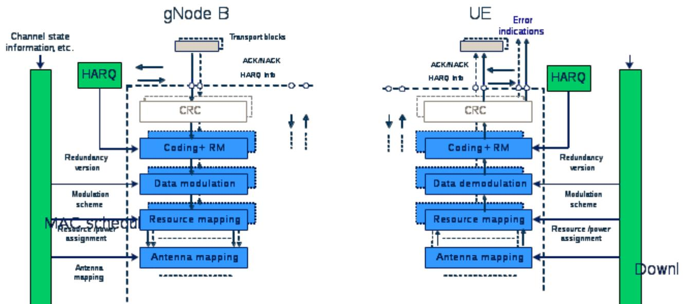
Figure 5.2.1-1: Physical-layer model for DL-SCH transmission
